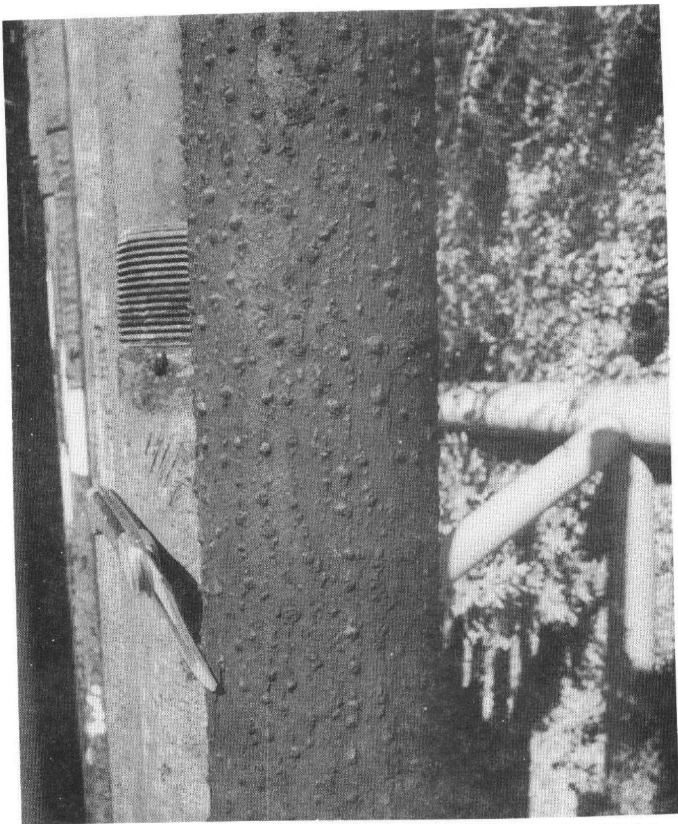
Figure 9.8 Corrosion of Section of Tubing Near Bottom of String from Remedial Treatment
