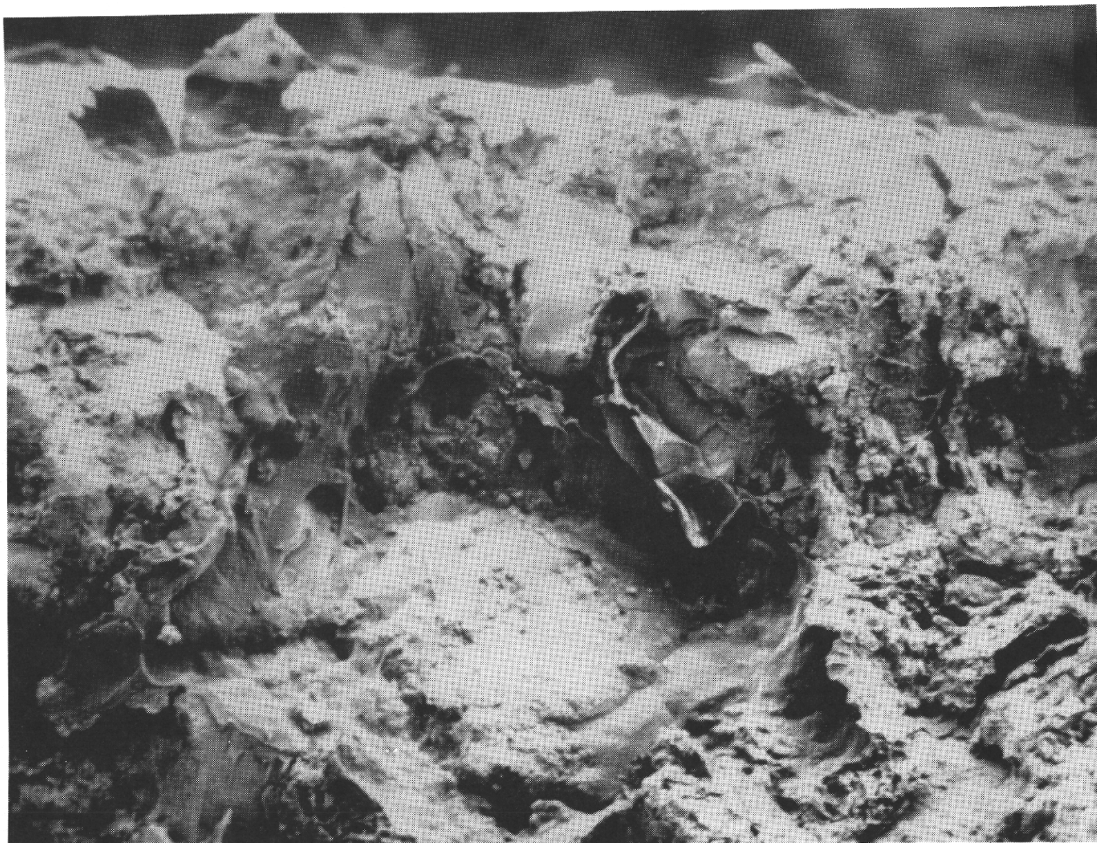
Figure 8.2 Dried Polymer on Crack Interior (Scale = 100 \mu\text{m} )
