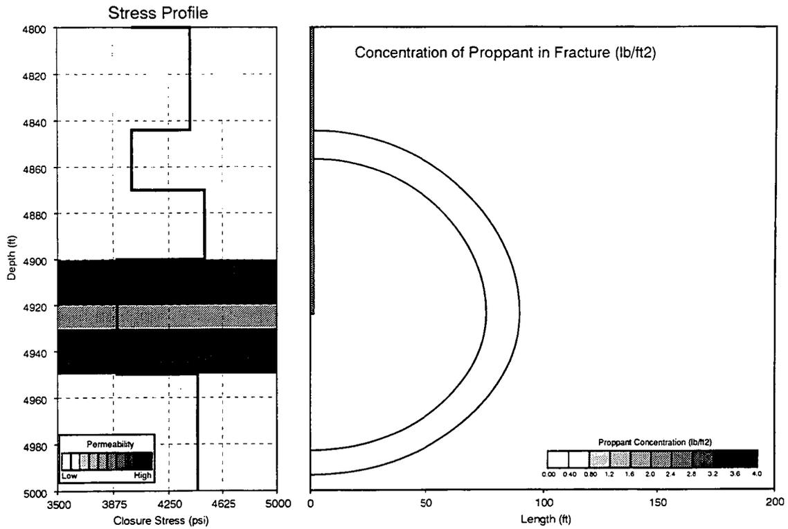
Figure 25 Stress Profile, Permeability Profile and Fracture Geometry for the KCl-Water Step-Rate Test
