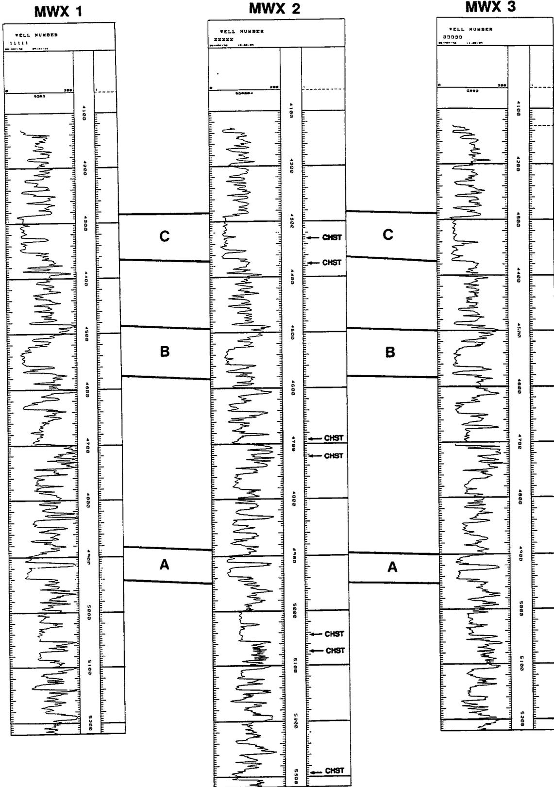
Figure 3 Upper Mesaverde Sandstone Units Proposed for M-Site No. 1 Research
