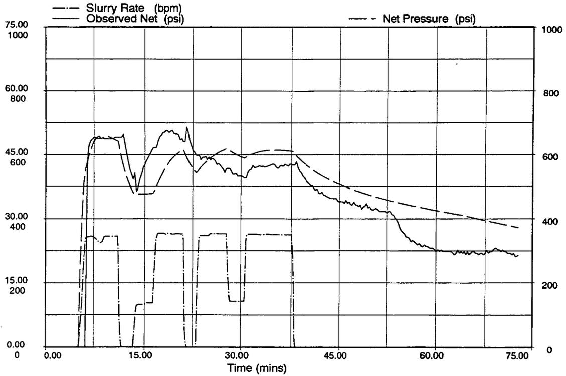
Figure 30 Net Pressure Match, Linear Gel Mini-Frac
