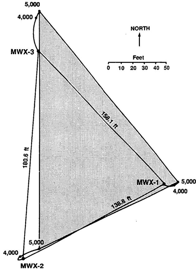
Figure 2 Closely-Spaced Wells of the MWX Project
