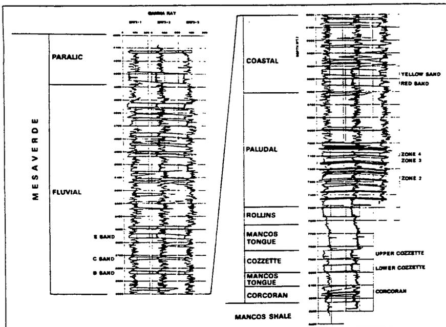
Fig. 2—Gamma ray logs of the three MWX wells through the Mesaverde Group showing the reservoirs tested.
