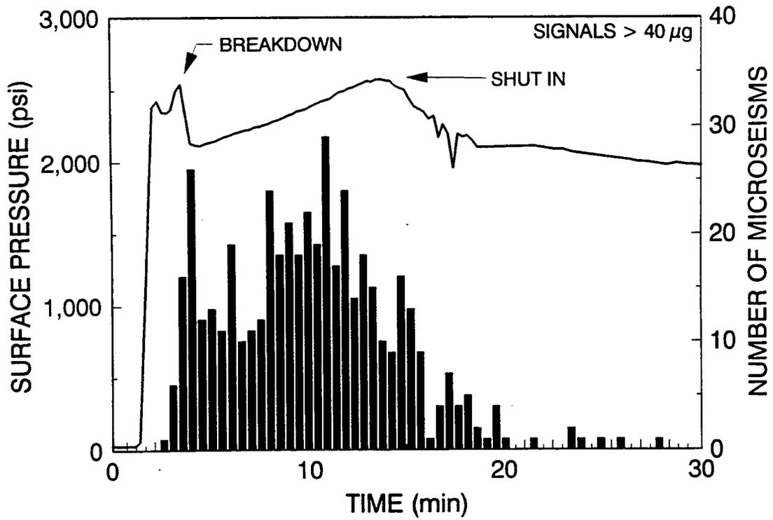
Figure 9 Histogram of Microseisms During Breakdown
