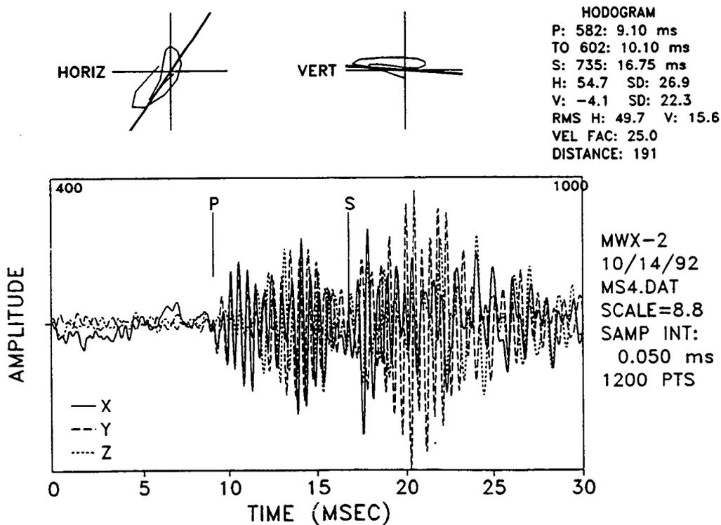
Figure 42 Overlay of Traces and Hodograms for Event No. 4, Unfiltered
