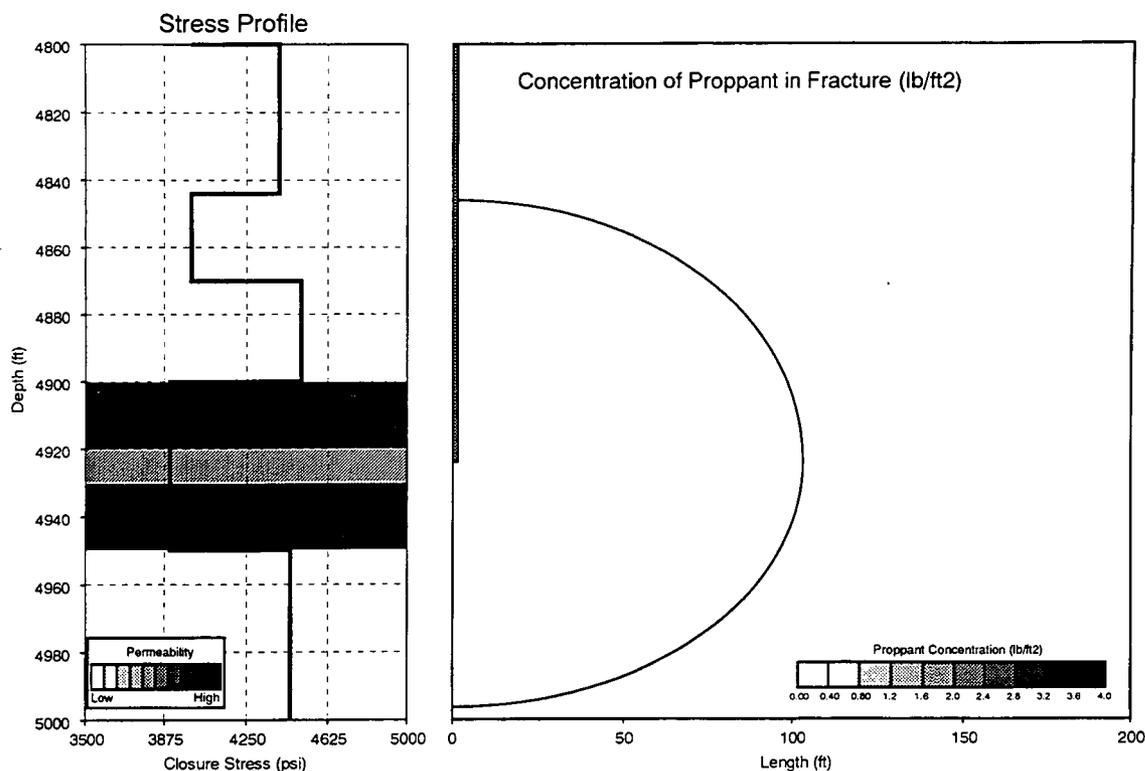
**Figure 22 Stress Profile, Permeability Profile and Fracture Geometry for the X-Linked Gel Ball-Out**
