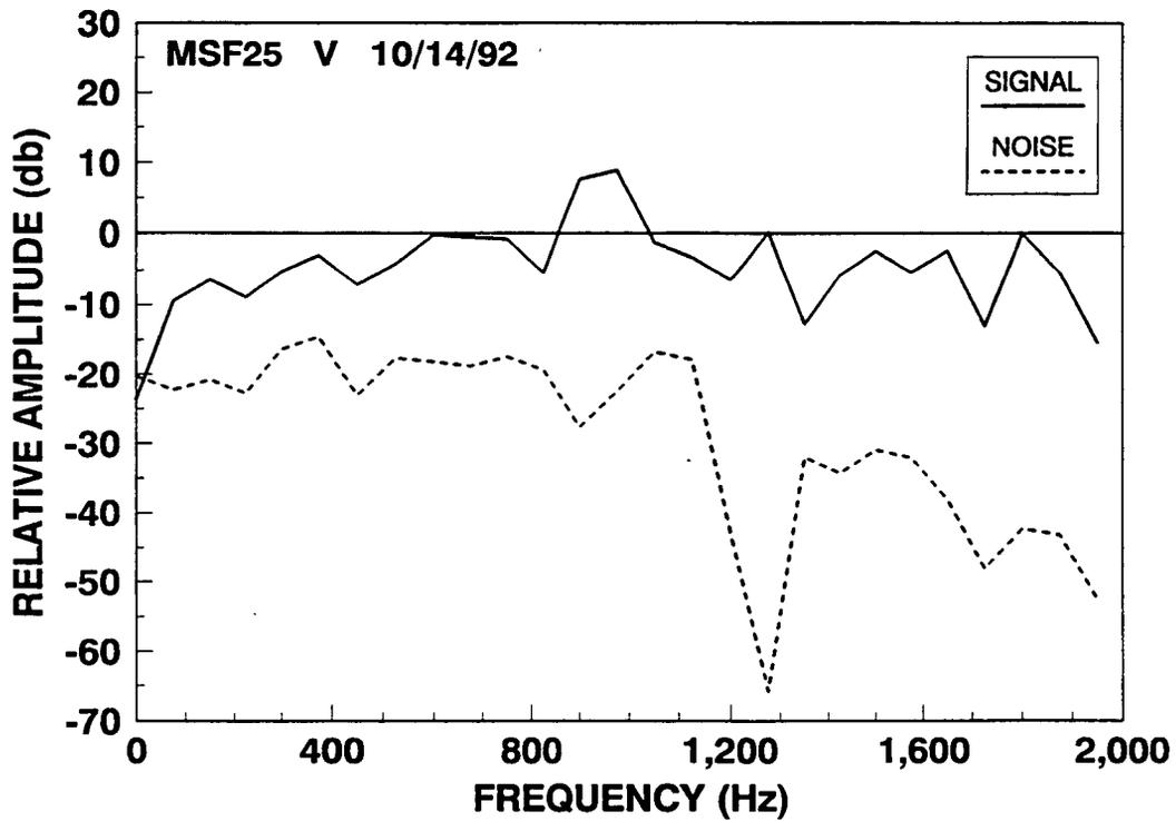
Figure 50 Noise and Signal Spectra, Event No. 25, Z Channel
