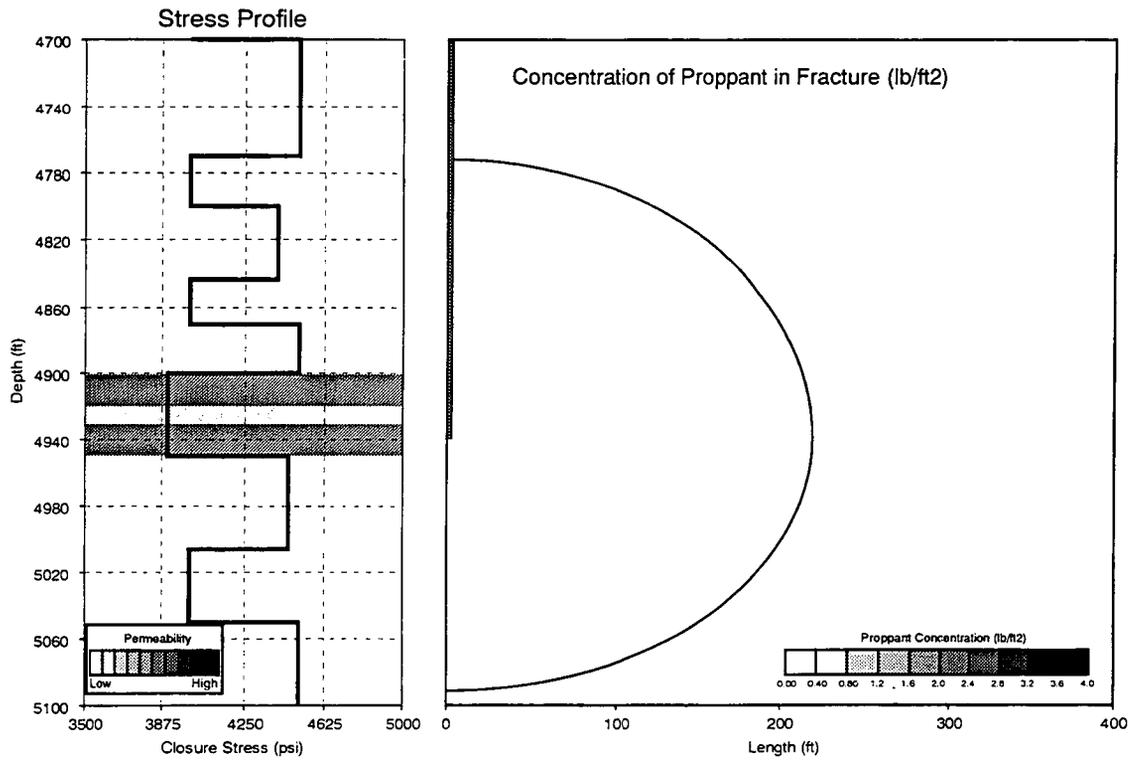
Figure 31 Stress Profile, Permeability Profile and Fracture Geometry for the Linear Gel Mini-Frac
