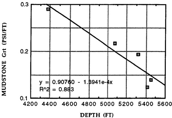
Figure 17 Mudstone Residual Tectonic Stress Gradient Versus Depth
