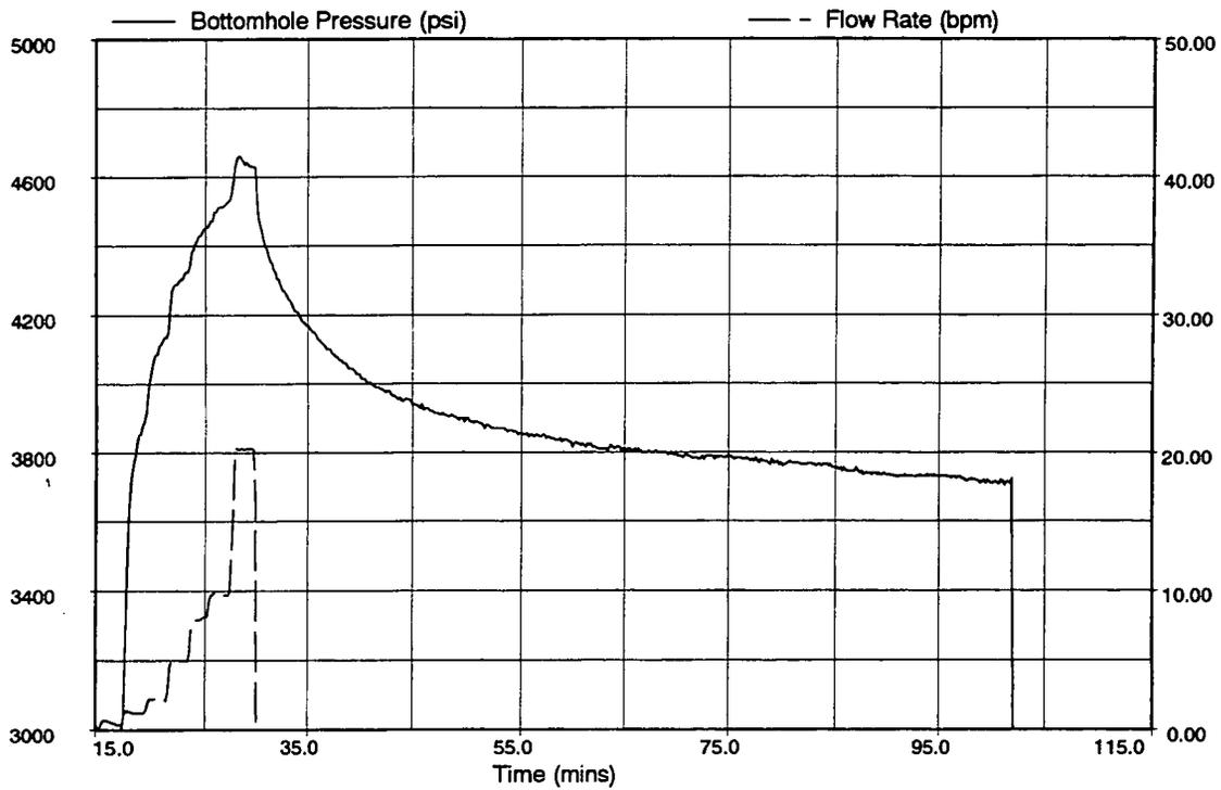
Figure 23 Treatment Data, KCl-Water Step-Rate Test
