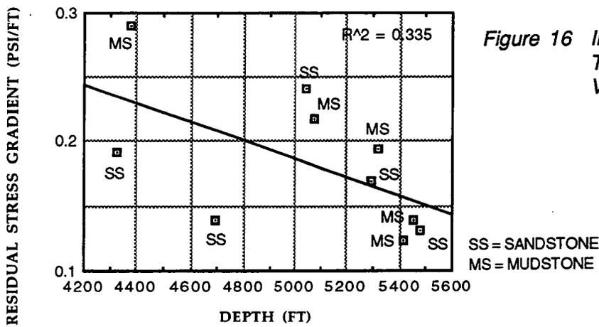
Figure 16 Interpreted Residual Tectonic Stress Gradient Versus Depth
