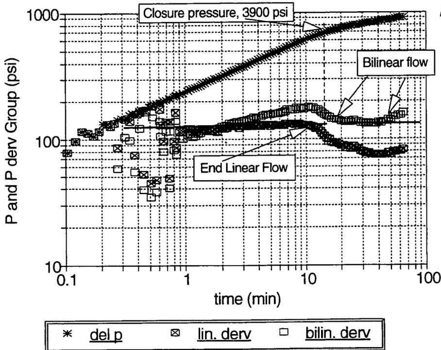
Figure 18 Log/Log and Derivative Group Plot of the Bottomhole Fall-Off Pressure Following the KCI Step-Rate Injection Test
