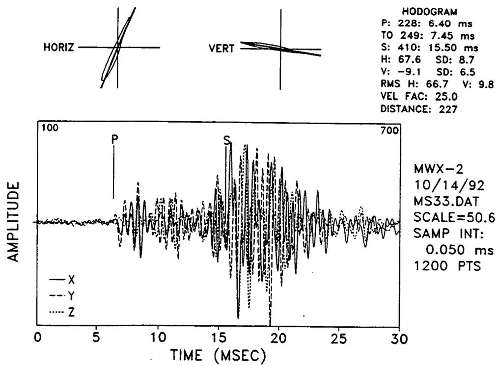
Figure 36 Overlay of Traces and Hodograms for Event No. 33, Unfiltered
