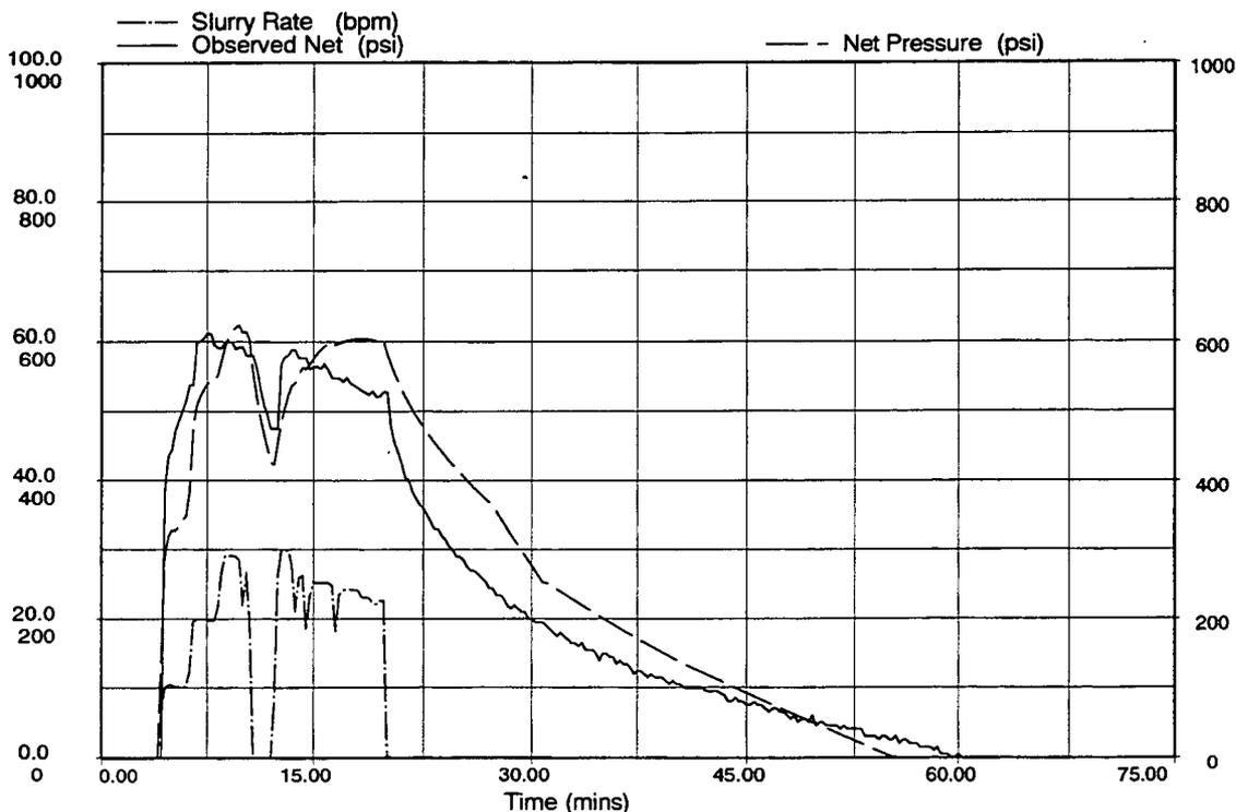
Figure 27 Net Pressure Match, KCI-Water Mini-Frac
