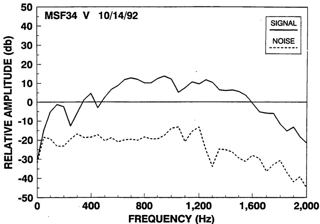
Figure 47 Noise and Signal Spectra, Event No. 34, Z Channel
