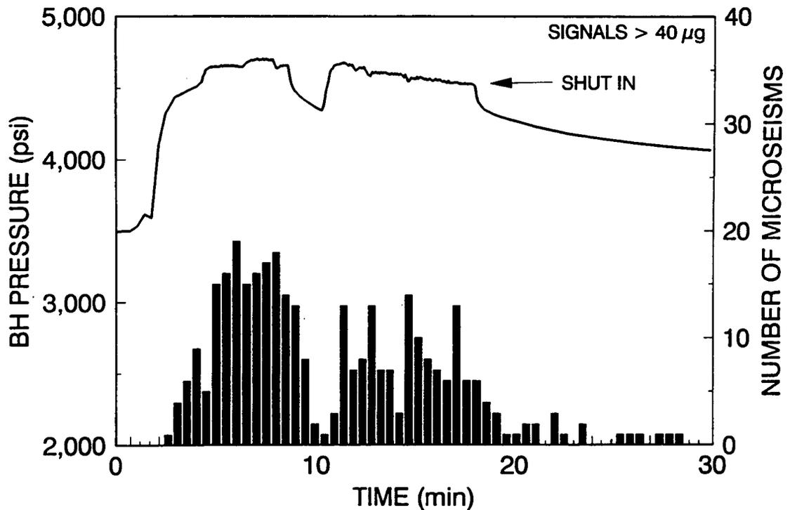
Figure 11 Histogram of Microseisms During KCl Mini-Frac
