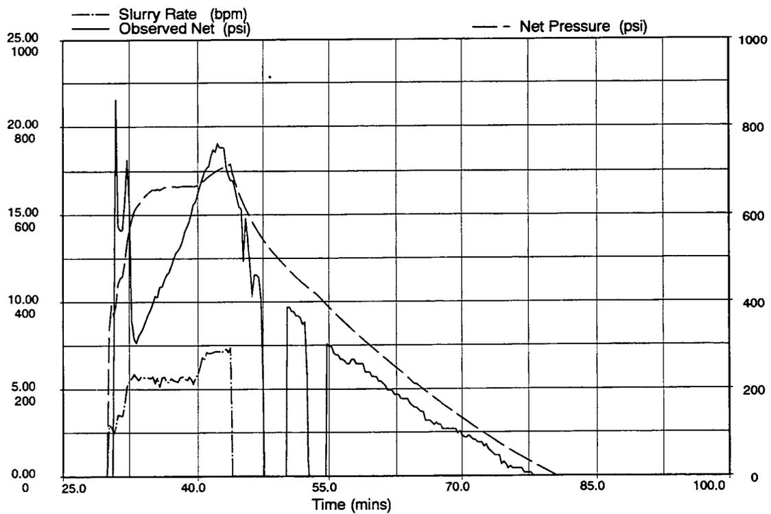
Figure 21 Net Pressure Match, X-Linked Gel Ball-Out
