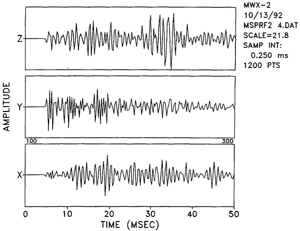
Figure 6 Example of Seismic Energy Generated from a Perforation Shot in MWX-2
