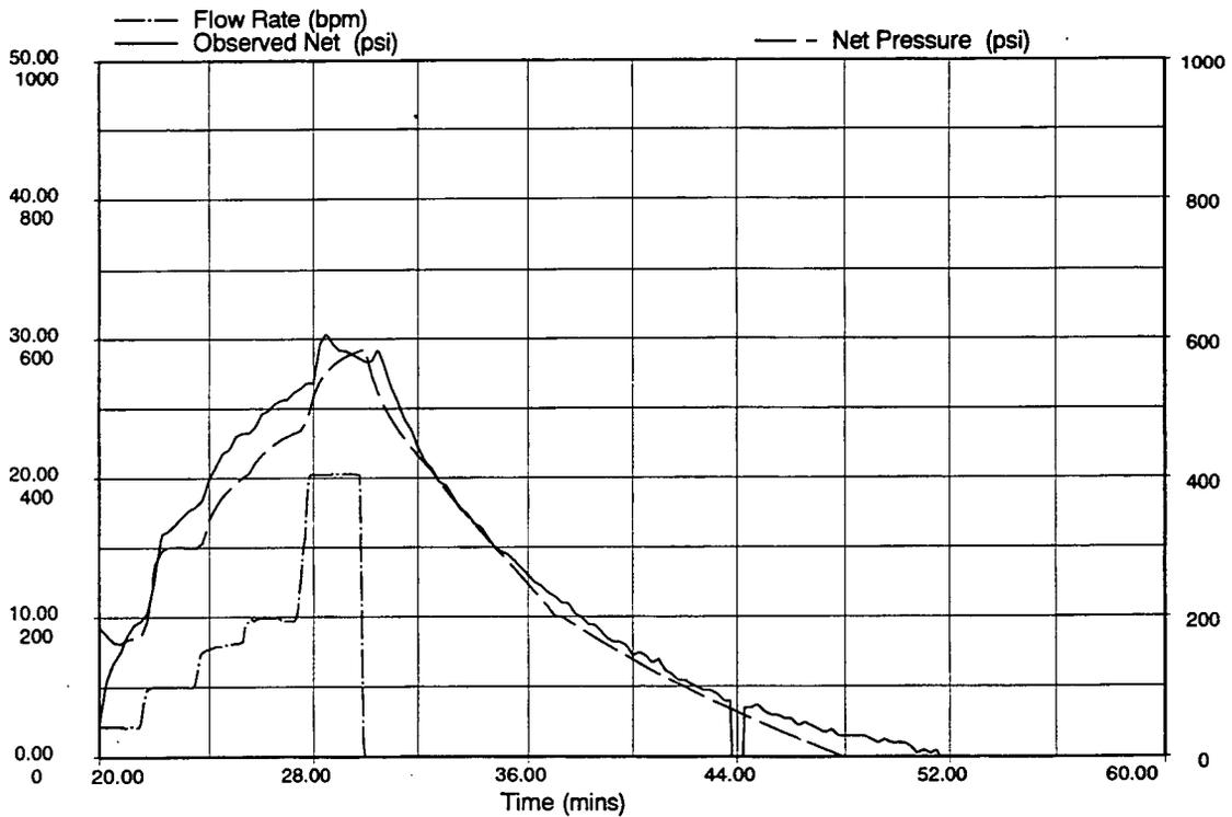
Figure 24 Net Pressure Match, KCl-Water Step-Rate Test
