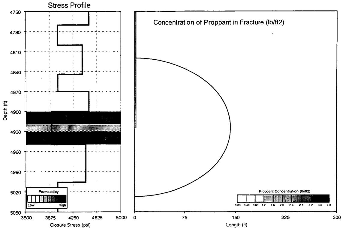
**Figure 28 Stress Profile, Permeability Profile and Fracture Geometry for the KCl-Water Mini-Frac**
