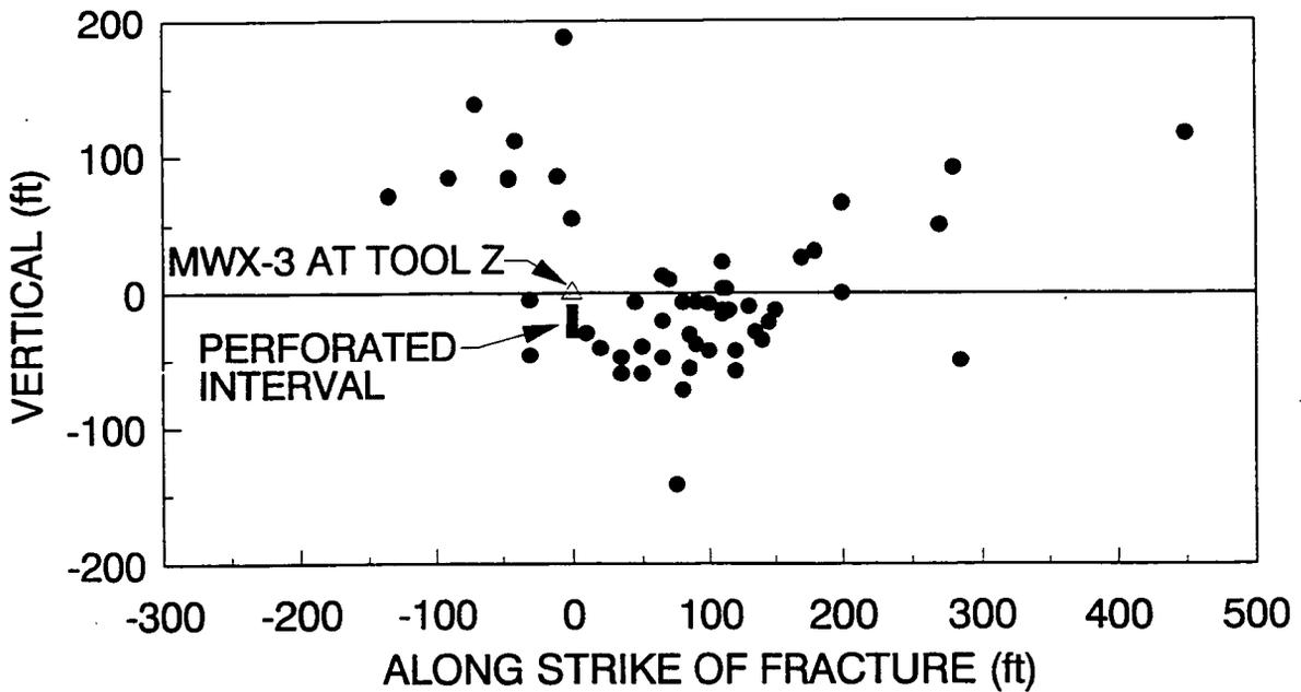
Figure 34 Side View of Microseism Map
