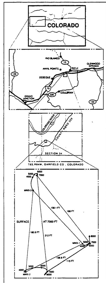
Fig. 1—Location of the MWX site and layout of the three MWX wells at the surface and at 7,000 ft.
