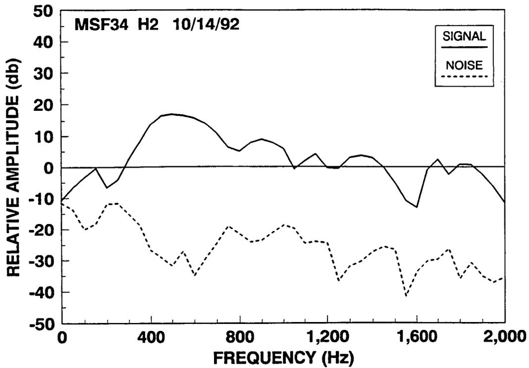
Figure 46 Noise and Signal Spectra, Event No. 34, Y Channel
