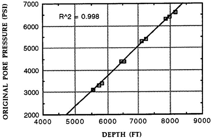
Figure 15 Original Pore Pressure Versus Depth
