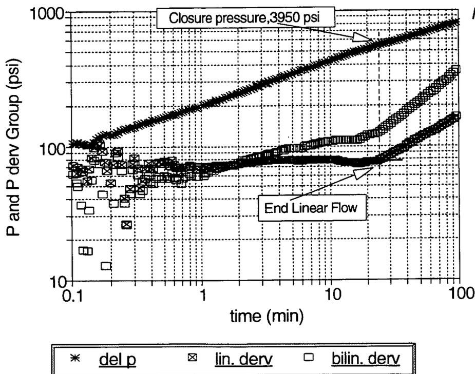
Figure 19 Log/Log and Derivative Group Plot of the Bottomhole Fall-Off Pressure. Following the KCI Mini-Frac Injection Test
