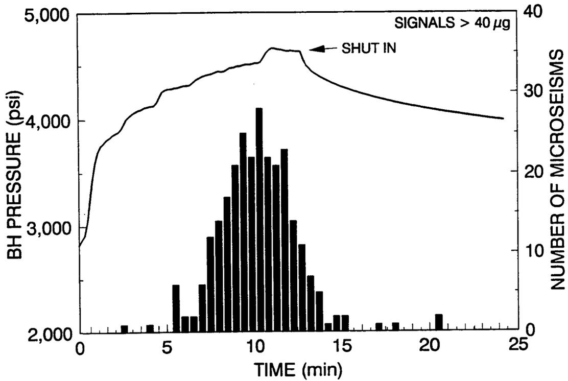
Figure 10 Histogram of Microseisms During Step-Rate Test
