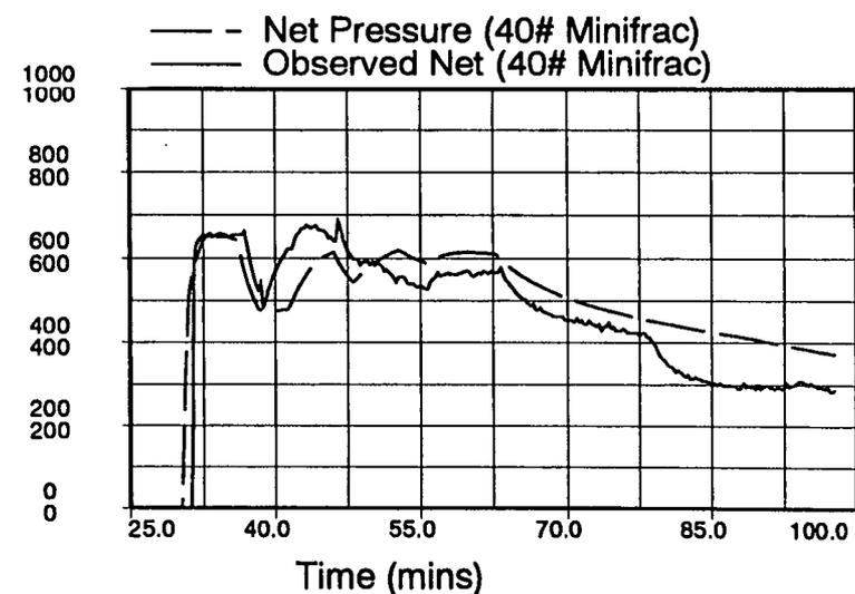
Figure 32 Net Pressure Matches, Comparison of All Injections
