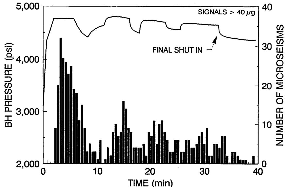
Figure 12 Histogram of Microseisms During Gel Mini-Frac
