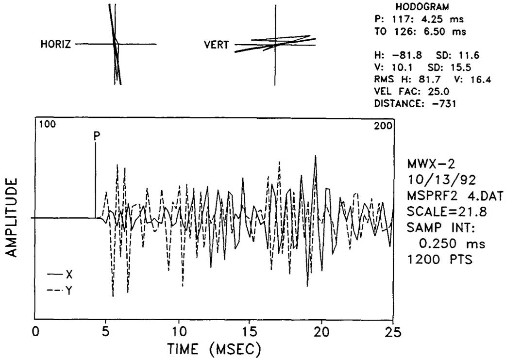
Figure 7 Overlay of X and Y Components and Hodogram, Perf Shot No. 1 in MWX-2
