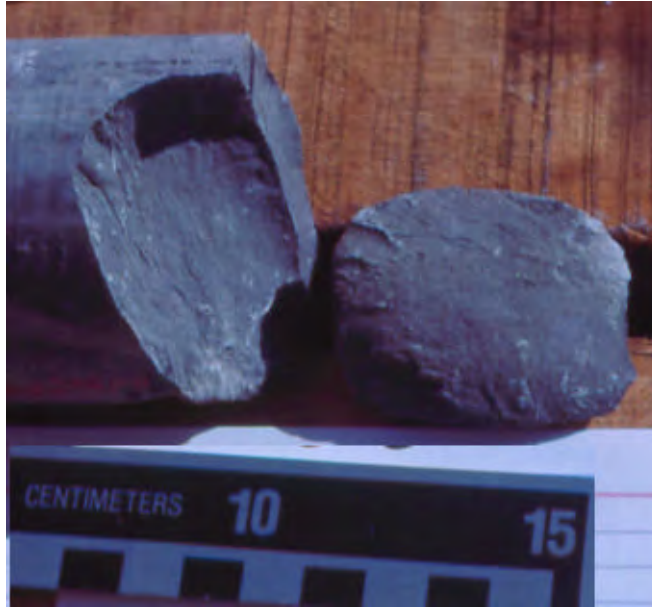
Figure 19. Drilling-induced petal fracture in siltstone of the Raton Formation. Stratigraphic top is to the left.
