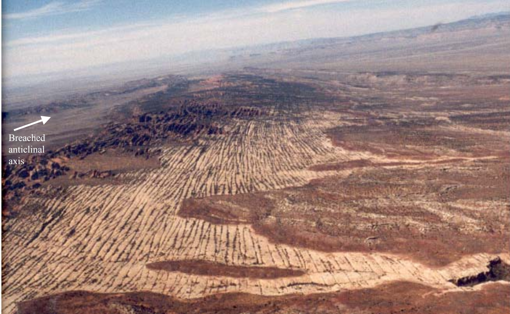
Figure 7A: Fracture domain B. Aerial photograph of fractures in domain B southeast of domain A. View is to the northwest, of a section of the northeastern anticlinal limb several km southeast of Figure 6A. Fractures here begin to fan out and strike up to 40° oblique to bedding strike. Figure 7B illustrates how these fractures are due to fan-wise extension normal to the axis of a plunging anticline.
