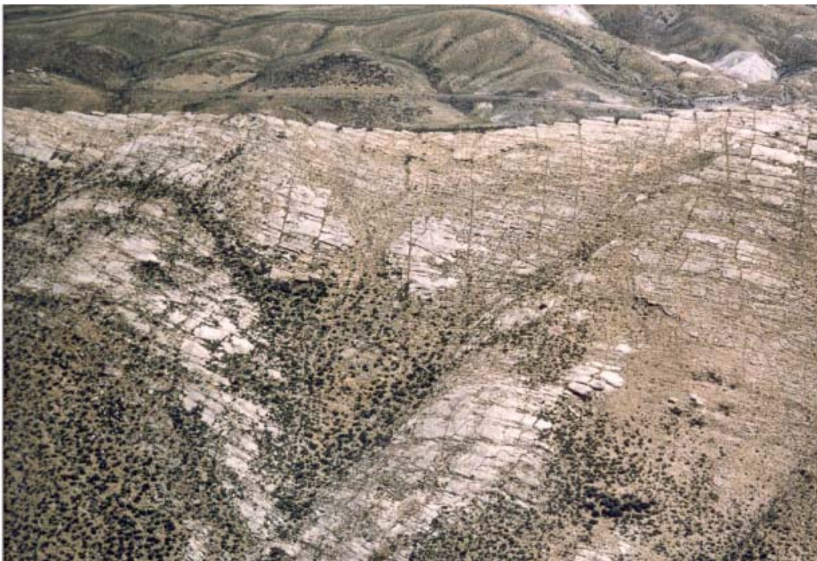
Figure 23: Aerial photograph illustrating the fracture pattern on a bedding-plane surface in a structurally simple area near the seismic road in Figure 22, wherein the oldest fractures are strike-parallel (horizontal across the photograph) and younger fractures are strike-normal (vertical across the photograph). View is to the east.
