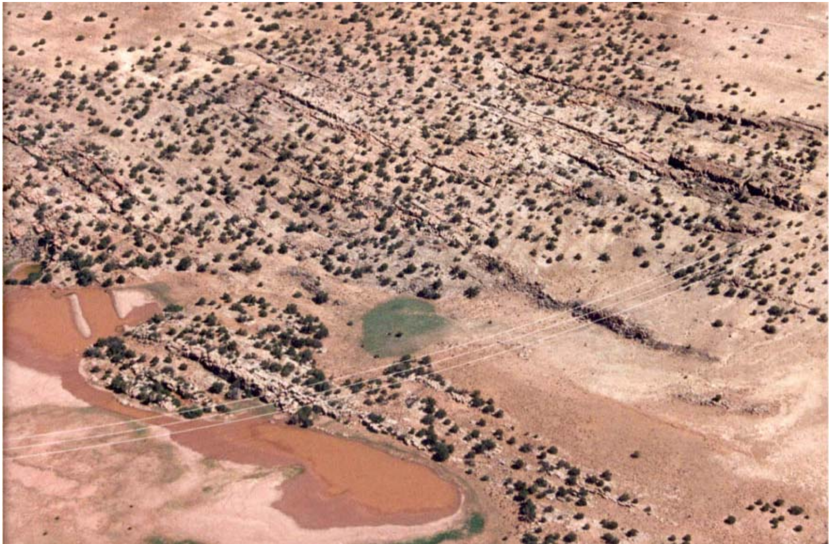
Figure 21: Aerial photograph of the Twin Lakes area on the southern limb of the Holbrook Anticline. Here the fractures are being widened and offset vertically by dissolution of the underlying strata.
