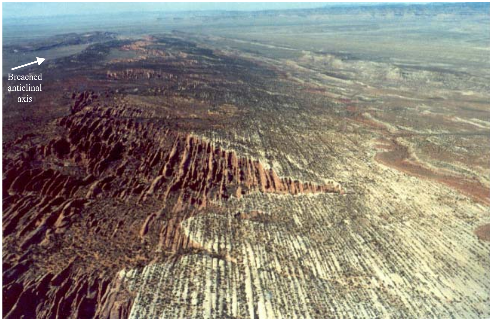
Figure 6A: Fracture domain A. Aerial photograph illustrating that fractures in the Entrada Sandstone of fracture domain A are parallel to the axis of the fold. View is to the northwest, along the northeastern limb of the anticline. Individual members of the Entrada Formation are identified by color with the dark red sandstone as the Slick Rock Member and the overlying light-gray to white sandstone as the Moab Member. Figure 6B illustrates how arching of strata over a rising salt core causes extensional fracturing parallel to the axis of the arch.
