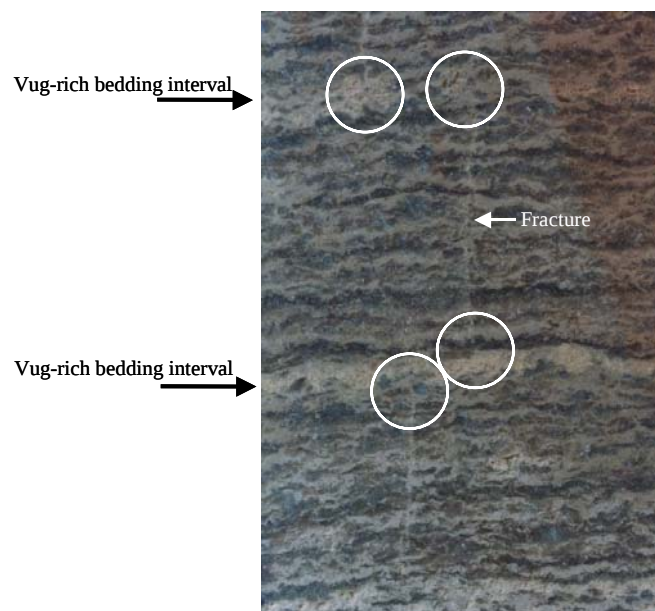
Figure 2.18. White circles denote areas where fractures within the Sulimar Queen core terminate at bedding intervals that contain vugs (i.e., intervals with vuggy porosity).
