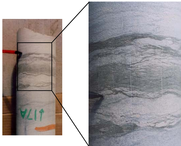
Figure 2.7. Layer of silty mudstone surrounded by sandstones of lithology A that is probably a large-scale permeability barrier (core section 17A, 4549 ft depth).
