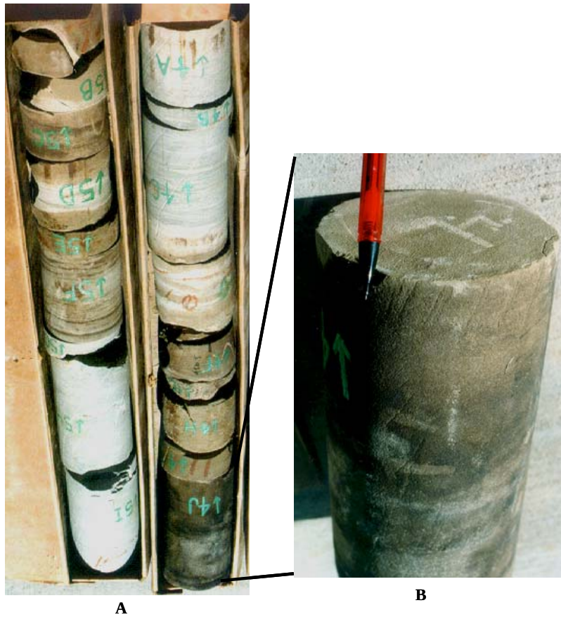
Figure 2.14. An abrupt color change between core section 4J (lower right hand corner of photo A) and the adjacent sections suggests invasive testing may have altered this section. B) Enlargement of core section 4J.
