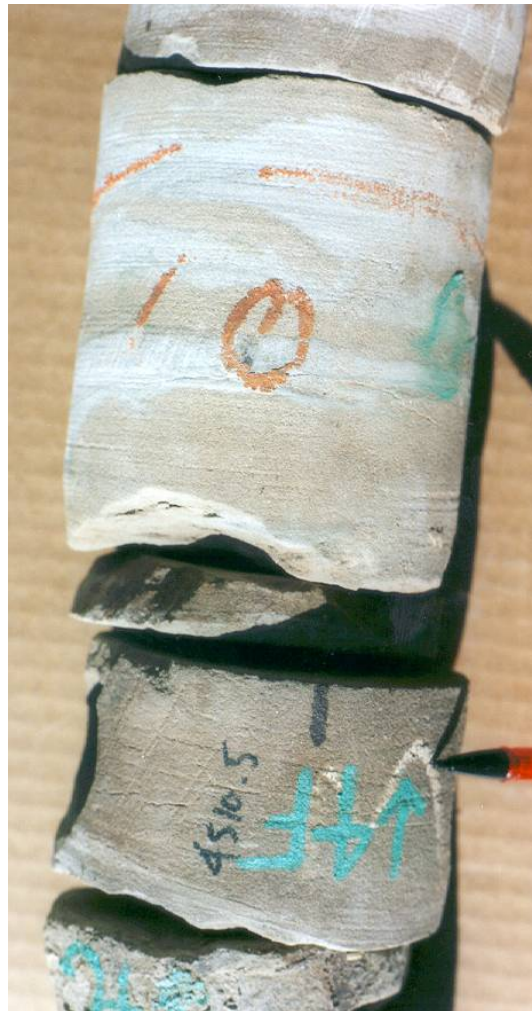
Figure 2.9. The massive and irregularly oil-stained nature of lithology C (core sections 4C, 4D, 4E, 4F, 4G, 4510.5 ft depth).
