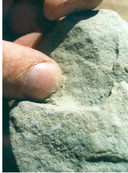
Figure 2.10. Portions of lithology C that are poorly cemented and friable—the rock disintegrates under minimum pressure.
