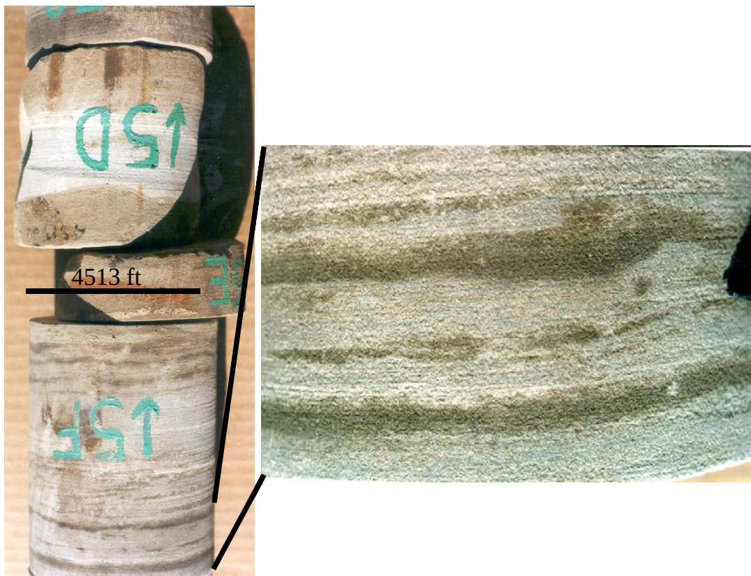
Figure 2.12. A heavily oil stained zone within lithology C near the 4513 ft mark. Enlarged photograph illustrates the bedding-parallel nature of the heaviest oil stain. This area is on the “backside” of core section 5F.
